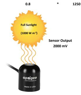
**Serial Number Range 0-10516.** Example of total shortwave radiation measurement with an Apogee SP-212 pyranometer. Full sunlight yields total shortwave radiation on a horizontal plane at the Earth's surface of approximately 1000 W m<sup>-2</sup> s<sup>-1</sup>. This yields an output signal of 2000 mV. The signal is converted to shortwave radiation by multiplying by the calibration factor of 0.5 W m<sup>-2</sup> per mV.
