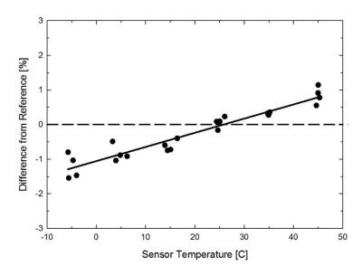
Mean temperature response of four Apogee silicon-cell pyranometers. Temperature response measurements were made at approximately 10 C intervals across a temperature range of approximately -10 to 50 C under sunlight. Each pyranometer had an internal thermistor to measure temperature. At each temperature set point, a reference blackbody pyranometer was used to measure solar intensity.
