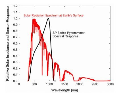
Spectral response of Apogee SP series pyranometers compared to solar radiation spectrum at Earth's surface. Silicon-cell pyranometers, such as Apogee SP series, are only sensitive to the wavelength range of approximately 350-1100 nm, and are not equally sensitive to all wavelengths within this range. As a result, when the spectral content of solar radiation is significantly different than the spectrum that silicon-cell pyranometers were calibrated to, spectral errors result.
